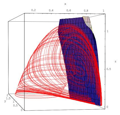
Fig. 4. Slow manifold surface based on the orthogonality principle and phase portrait of the Volterra-Gause system (12) with the same parameter values. In this figure, we can see the slow manifold on which the solutions of the system (12) are based.
