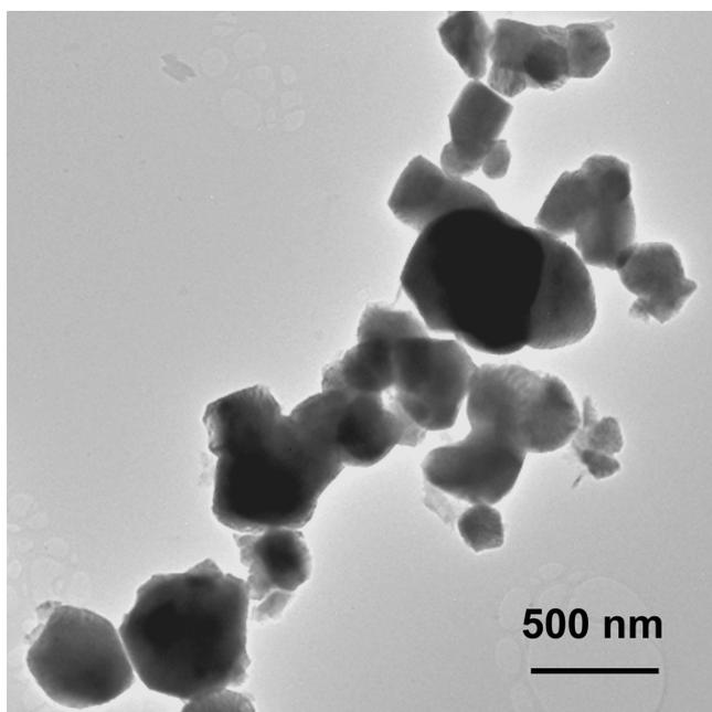
The  $\text{Co}_x\text{Fe}_{3-x}\text{O}_4$  pellets used for impedance spectroscopy were characterized by XRD and TEM coupled to EDS. During the electrical impedance spectroscopy measurements, these pellets were heated up to  $900^\circ\text{C}$ , thus were liable to possible phase transitions and grain growth. Fig.2 shows typical grains of the pellets heated up to  $900^\circ\text{C}$ .
