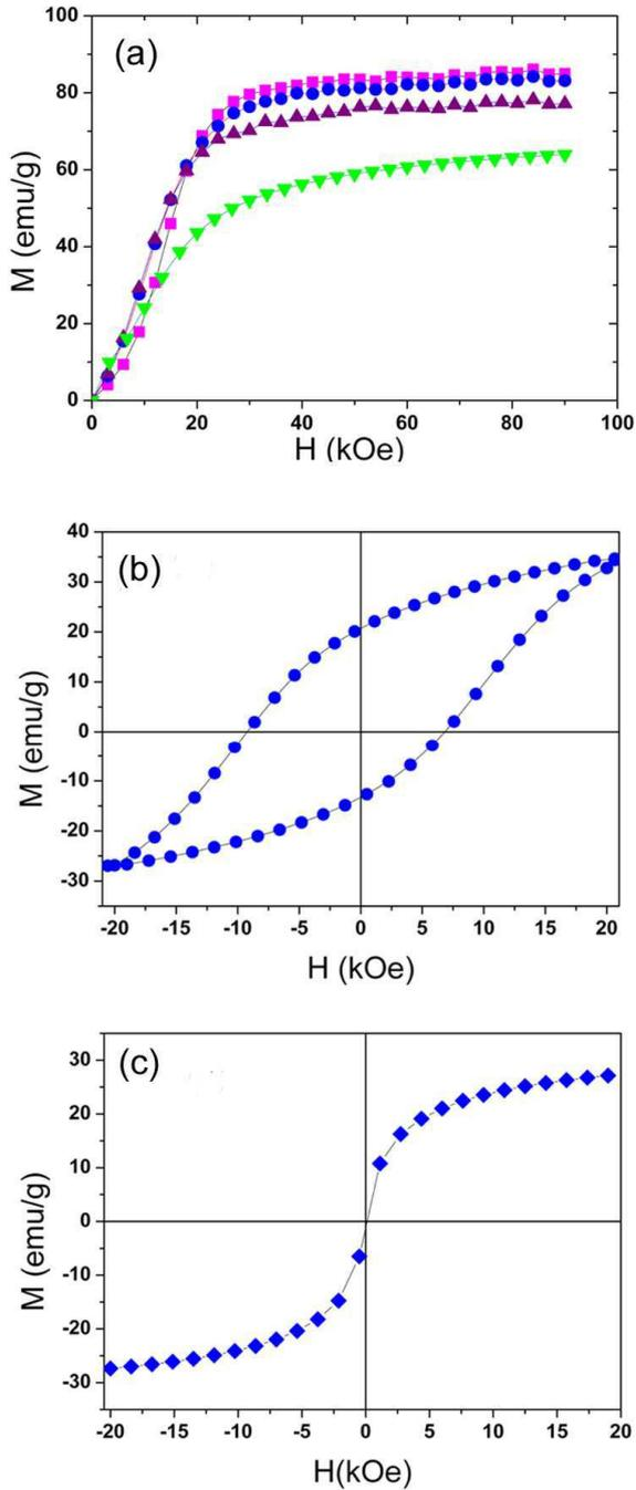
Figure 6: a) Magnetization versus applied field at 10K for  $Co_xFe_{3-x}O_4$  powders  $x=0.6$  ( $\square$ ),  $x=1$  ( $\circ$ )  $x=1.2$  ( $\nabla$ ) and  $x=1.8$  ( $\Delta$ ), b) and c) Magnetization curves for  $Co_{1.8}Fe_{1.2}O_4$  under medium H field at two temperatures: b) 10 K, c) 300 K.
