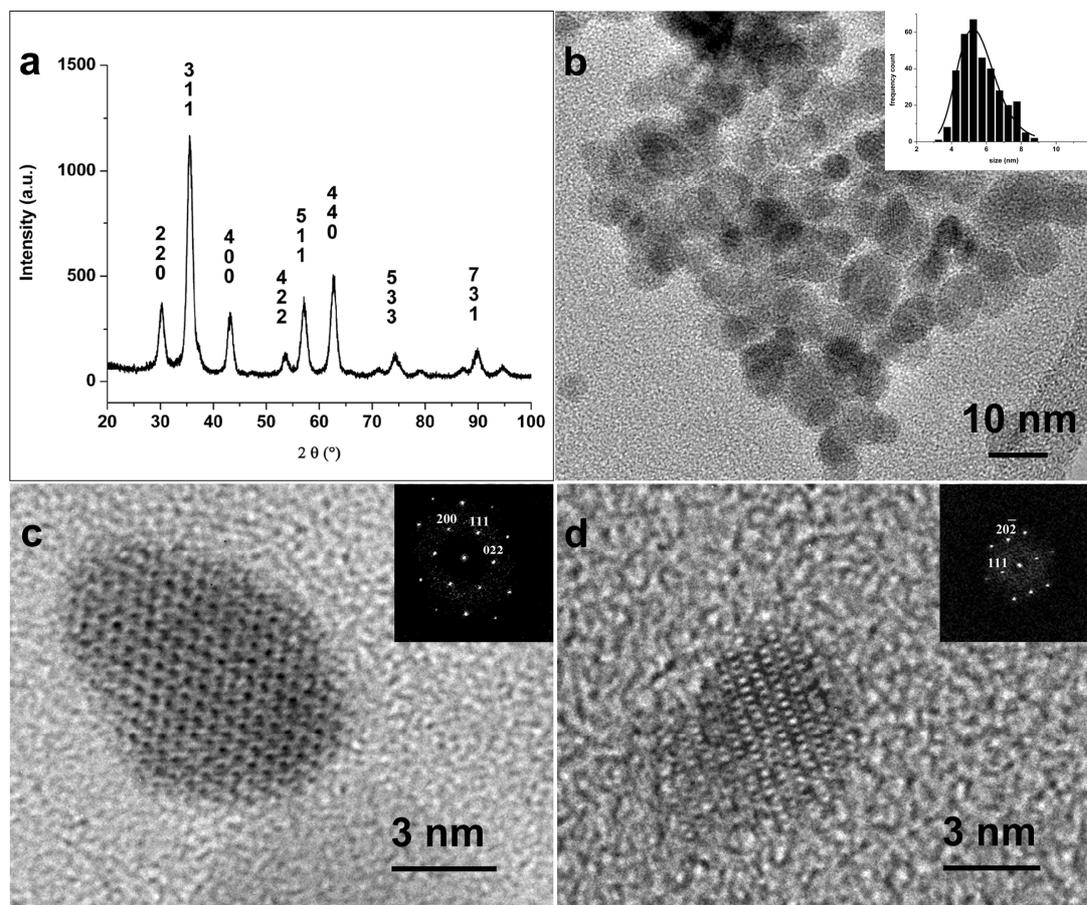
Figure 1: a) X rays diagram of the  $\text{Co}_{1.2}\text{Fe}_{1.8}\text{O}_4$  nanopowder, indexed in the spinel structure, b) TEM image of  $\text{Co}_{1.2}\text{Fe}_{1.8}\text{O}_4$  nanoparticles, along with the size distribution. c) and d) HRTEM images of single cobalt ferrites nanoparticles, c)  $\text{CoFe}_2\text{O}_4$  oriented along  $[01\bar{1}]$  (see FFT) and d)  $\text{Co}_{1.8}\text{Fe}_{1.2}\text{O}_4$  oriented  $[\bar{1}21]$  (see FFT).
