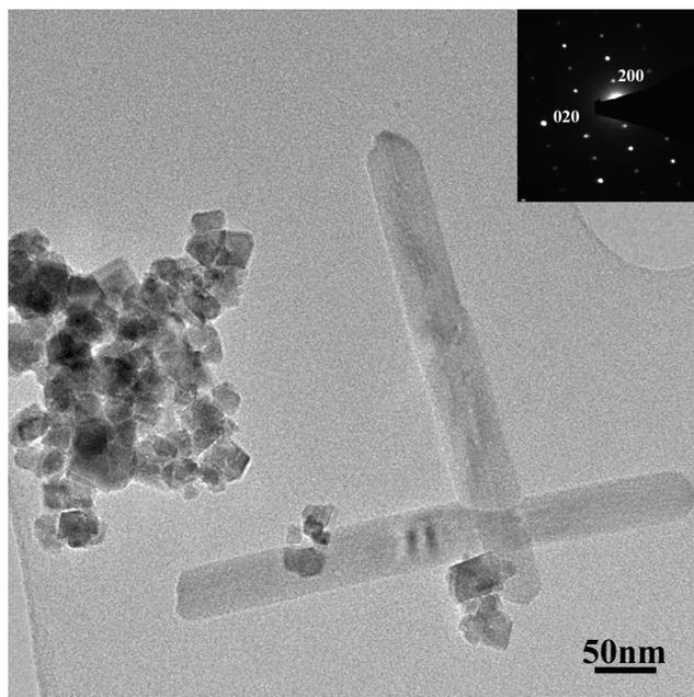
*Fig. 2 TEM image of  $\text{CoFe}_2\text{O}_4$  nanoparticles and goethite rods. The electron diffraction pattern of one rod like grain was indexed in the goethite structure with a  $[001]$  zone axis (inset)*
