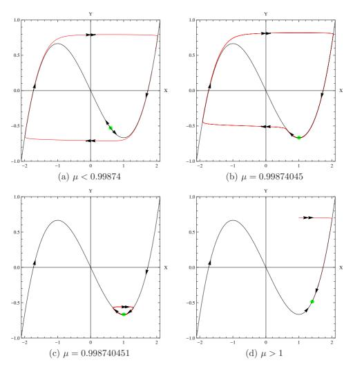
FIGURE 1. Transition from relaxation oscillation to canard explosion.
