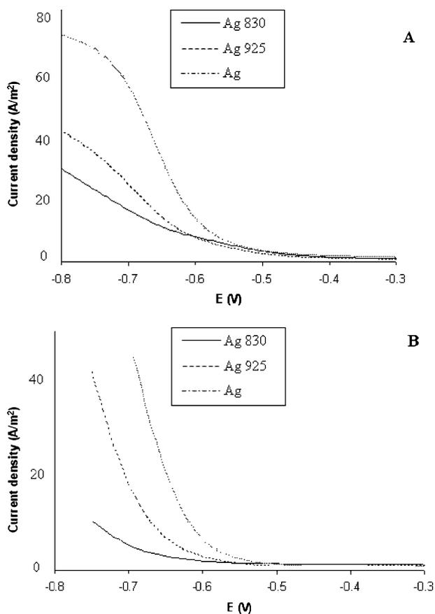
**Fig. 1** Linear scan of pure silver, silver 830 and silver 925 in **a**  $\text{HNO}_3$  ( $0.01$  M) and **b**  $\text{HCl}$  ( $0.1$  M). Scan rate was  $15$  mV s $^{-1}$ , and the scan was performed after a  $5$ -s resting time
