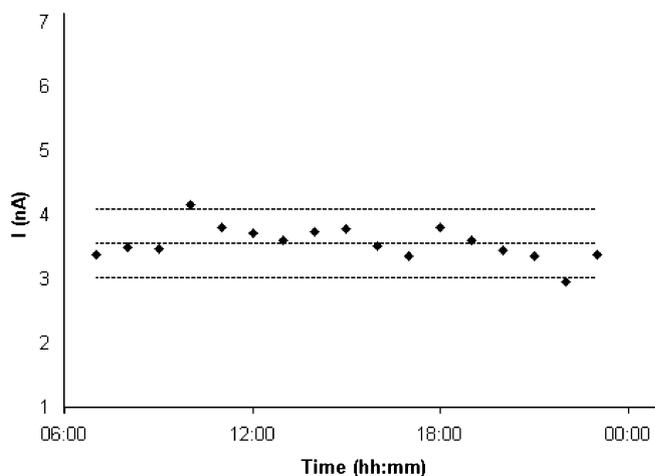
**Fig. 10** Repeatability test in real sample from the river Deûle. Peak heights for zinc are plotted as a function of time. Repetitive measurements in the same sample during a period of 16 h using differential pulse stripping voltammetry with a deposition time of 240 s at  $-1,250$ , a scan rate of  $15 \text{ mV s}^{-1}$  and a modulation pulse of 75 mV. Upper and lower horizontal lines indicate  $2 \times$  standard deviation
