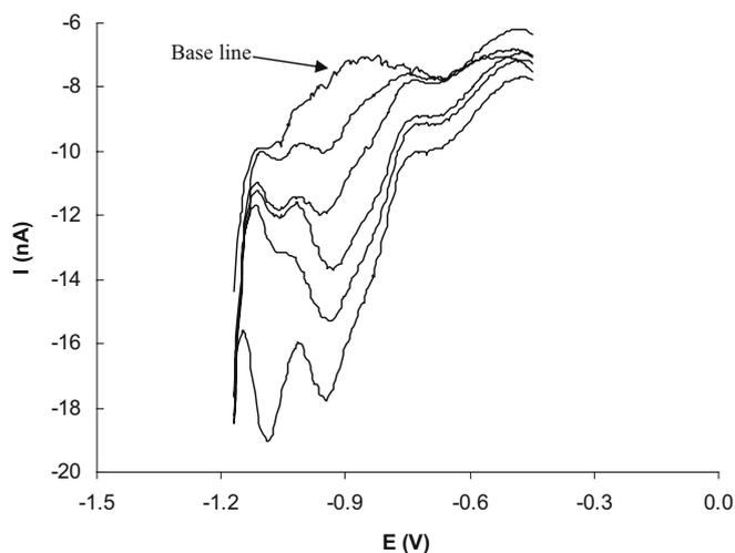
**Fig. 8** Standard additions of  $3.2$ ,  $6.5$ ,  $13$  and  $26$  mg L $^{-1}$  nitrate and then  $5$   $\mu$ g L $^{-1}$  nickel in ammonium buffer solution (pH 8.6). Differential pulse voltammetry scanning from  $-450$  mV to  $-1,200$  mV with a scan rate of  $15$  mV s $^{-1}$ , and a modulation pulse of  $-75$  mV
