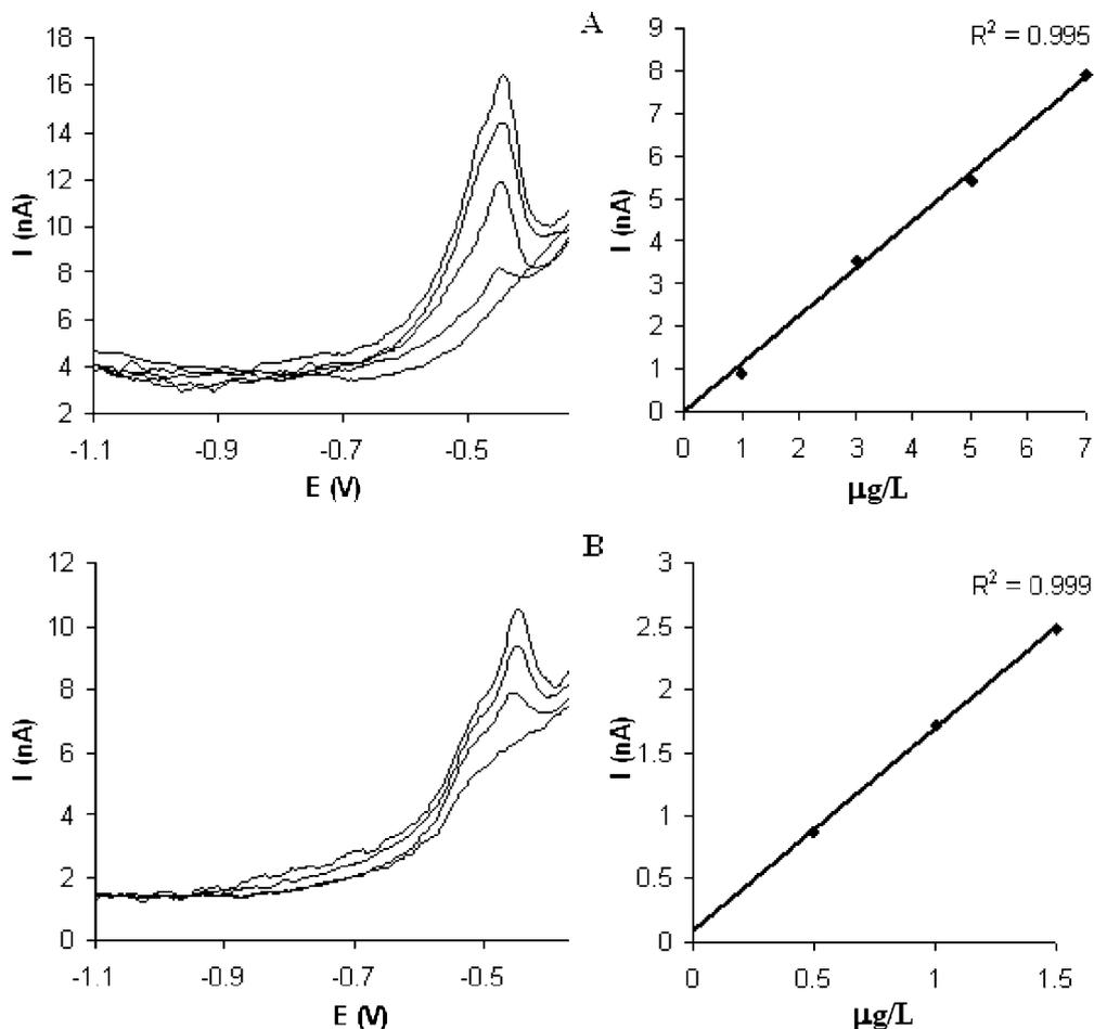
**Fig. 5** DPASV of standard additions of lead **a** 1, 2, 3, 5, 7, 10  $\mu\text{g L}^{-1}$ ) and **b** 0.5, 1, 1.5, 2, 2.5  $\mu\text{g L}^{-1}$  in ultrapure water using a silver electrode containing 17% added copper. The scan rate was  $15 \text{ mV s}^{-1}$ , modulation pulse 70 mV and deposition time were 600 s (a) and 1,200 s (b) at  $-1,250 \text{ mV}$ . Relative standard deviation was 2.5% ( $n=5$ )
