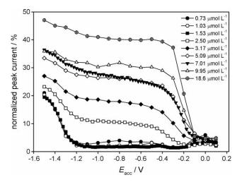
**Fig. 2.** Pseudopolarograms of interest obtained by DPASV for logarithmic copper additions on the concentrated sample (pH = 8.2) represented as the fraction of measured electro-active copper (compared to total added copper) as a function of deposition potential.  $t_{\rm dep}$  = 297 s at  $E_{\rm dep}$  (from -1.5 V to 0.1 V) + 3 s at  $E_{\rm dep2}$  = -1.6 V.
