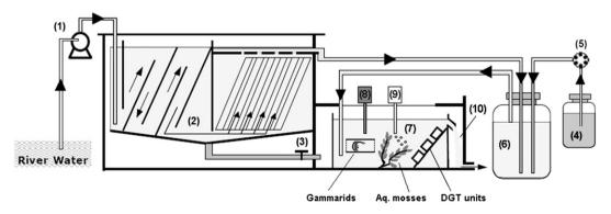
**Fig. 1.** Exposure system composed of a pump set at 0.5 L min<sup>-1</sup> (1), a lamellar decanter (2), a purge valve (3), a 6 L Cu stock solution (10 or 30 mg L<sup>-1</sup>) (4), a peristaltic pump set at 0.25 mL min<sup>-1</sup> (5), a 20 L reservoir for Cu-contaminated water (6), a 20 L tank (7), a multi-parameter probe (8), an aeration system (9) and a system overflow (10). Adapted from (Ferreira et al., in press).
