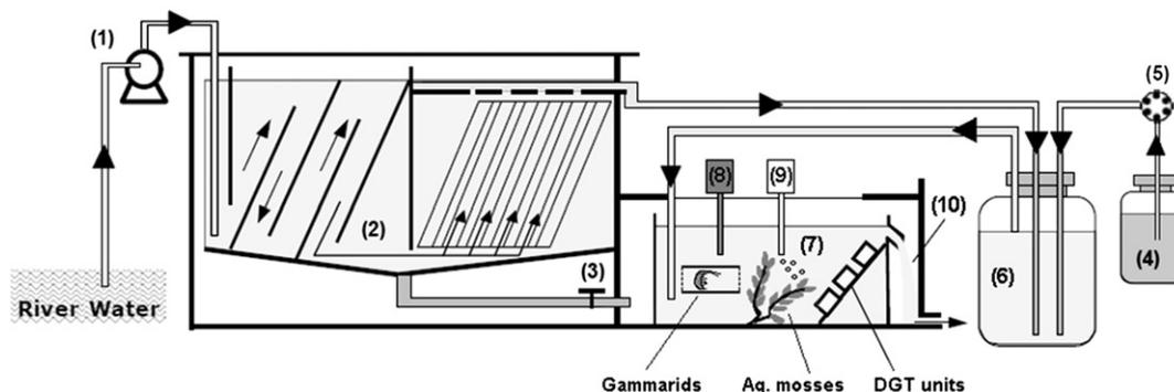
**Fig. 1.** Exposure system composed of a pump set at  $0.5 \text{ L min}^{-1}$  (1), a lamellar decanter (2), a purge valve (3), a 6 L Cu stock solution ( $10$  or  $30 \text{ mg L}^{-1}$ ) (4), a peristaltic pump set at  $0.25 \text{ mL min}^{-1}$  (5), a 20 L reservoir for Cu-contaminated water (6), a 20 L tank (7), a multi-parameter probe (8), an aeration system (9) and a system overflow (10). Adapted from (Ferreira et al., in press).
