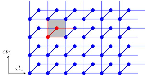
Figure 12: Planar structure leading to Cosserat model.
