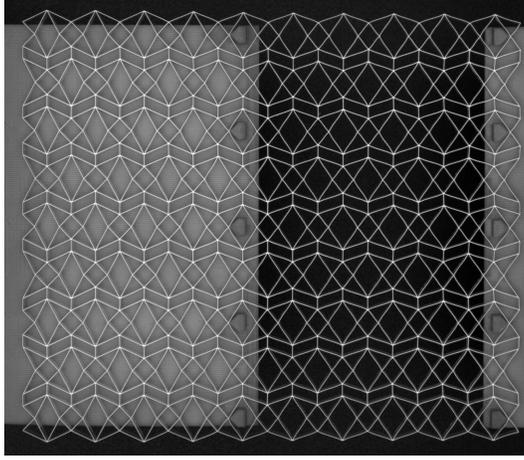
Figure 11: Experiment : traction of a pantographic membrane.
