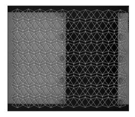
Figure 13. Experiment: traction of a pantographic membrane.
