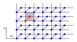
Figure 14. Planar structure leading to Cosserat model.
