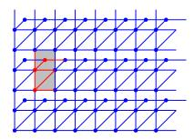
**Figure 15.** Planar structure leading to both second gradient and Cosserat effects.
