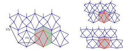
**Figure 12.** Pantographic membrane and its two admissible deformations (bending of the bars are not represented in the deformed configurations).
