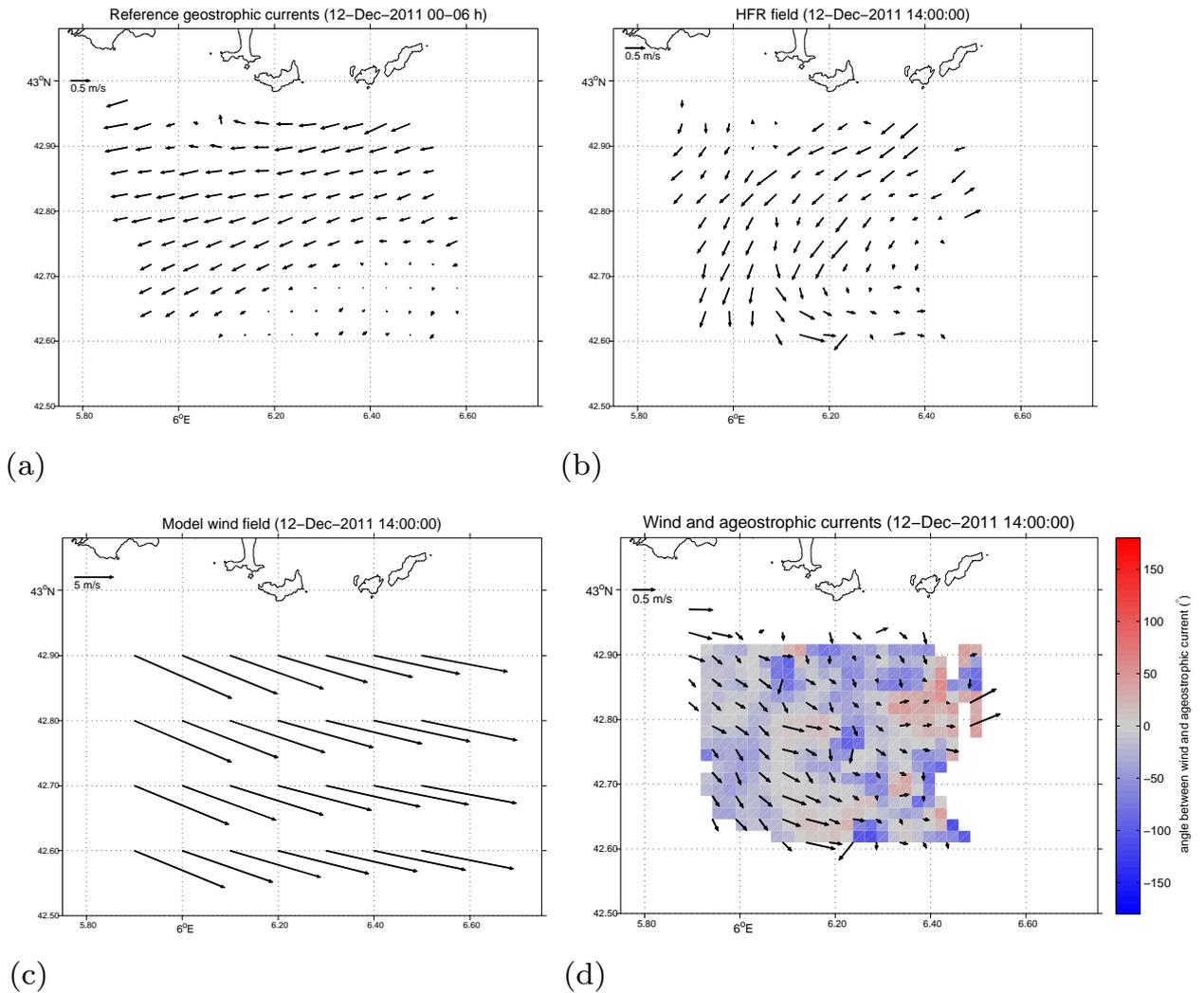
**Figure 11.** Example maps of: (a) 6h time-averaged geostrophic flow  $\mathbf{u}_{Sg}$  derived from HFR, (b) instantaneous HFR surface currents  $\mathbf{u}_S$ , (c) ALADIN wind field, and (d) ageostrophic surface currents  $\mathbf{u}_{S\alpha W}$  superimposed on the color coded map quantifying the angle  $\alpha$  between the ageostrophic component and ALADIN wind. Negative values means current to the right of the wind.
