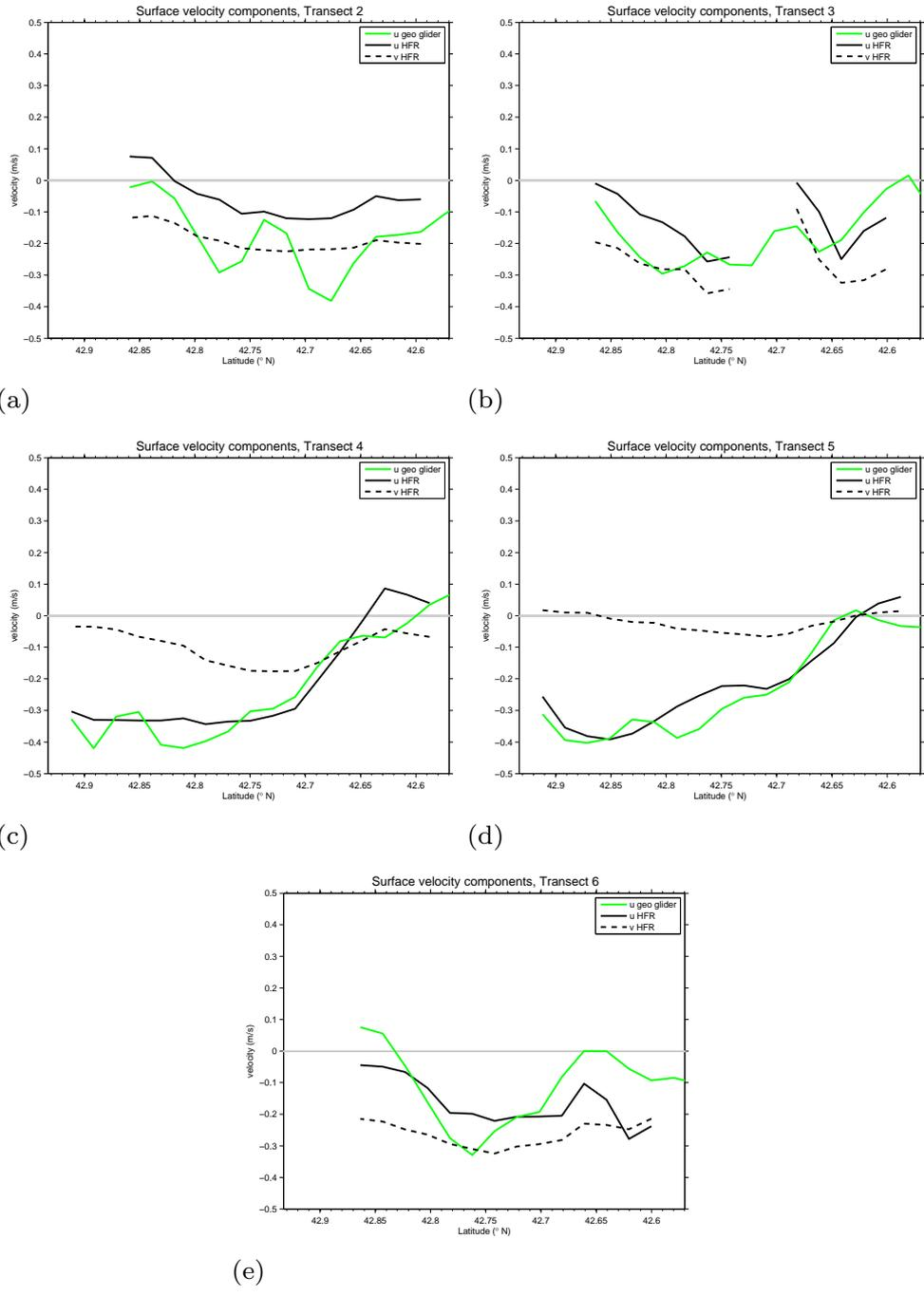
**Figure 9.** Comparison of  $u_S$  (solid black line) and  $v_S$  (dashed black line) components of total surface currents from HFR and  $u_{Sg}$  (green line) geostrophic component from glider transects. Positive  $u$  ( $v$ ) currents are eastward (northward), and the gray line indicates null velocities. Panels (a) to (e) represent measurements during Transects 2 to 6.
