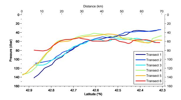
Figure 7. Potential density anomaly  $\sigma(z)$ =28.7 kg/m<sup>3</sup> isopycnal evolution color coded for each glider transect.
