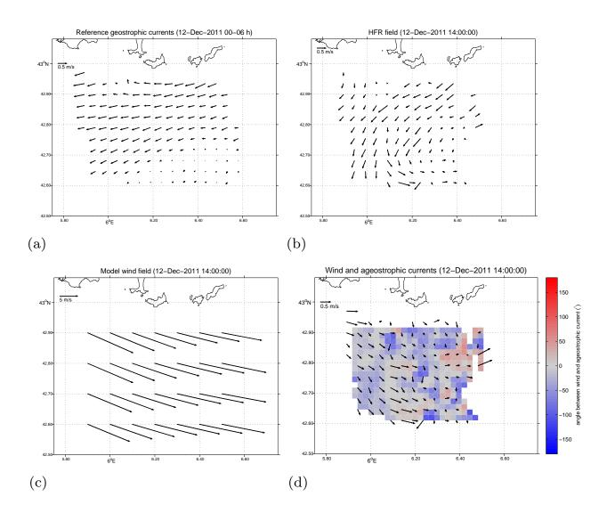
Figure 11. Example maps of: (a) 6h time-averaged geostrophic flow  $\mathbf{u}_{Sg}$  derived from HFR, (b) instaneous HFR surface currents  $\mathbf{u}_{S}$ , (c) ALADIN wind field, and (d) ageostrophic surface currents  $\mathbf{u}_{SaW}$  superimposed on the color coded map quantifying the angle  $\alpha$  between the ageostrophic component and ALADIN wind. Negative values means current to the right of the wind.
