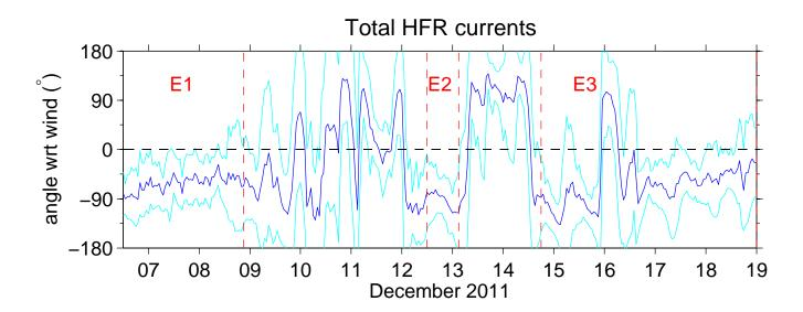
Figure 10. Angle  $\bar{\alpha}(t)$  between total surface currents  $\mathbf{u_S}$  and average ALADIN winds over the HFR coverage (blue line). Negative angles indicate currents to the right of the wind direction. The cyan lines represent the std. The limits of the selected wind events (E1, E2, and E3) are indicated with red dashed lines (see Fig. 2b for more details).
