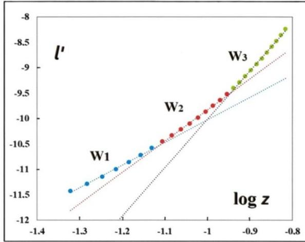
Fig. 9. Variation of  $l'$  vs  $\log z$  for  $\text{Fe}_{1-z}\text{O}$  at  $1250\text{ }^\circ\text{C}$ . Three sets of data can be defined as three quasi-linear relations.
