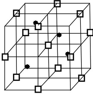
**Fig. 13: The Koch and Cohen cluster (13:4) associated with a 3X commensurate structure of wüstite  $\text{Fe}_{0.902}\text{O}$ .**
