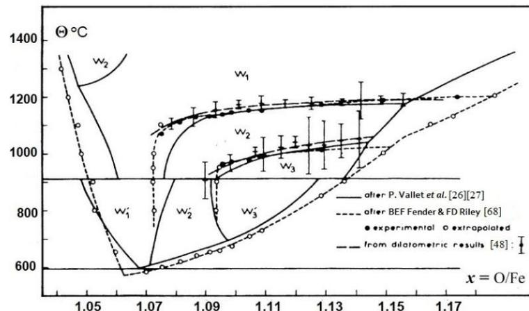
**Fig. A2. Comparative plot of experimental phase diagram versions (from ref. [50]) by Vallet and Racciah [26] and Fender and Riley [67].**
