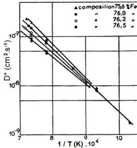
Fig. 11: Fe diffusion (from ref. [112], Fig.4) :  $\log D_{\text{Fe}}^*$  vs  $1/T$ .
