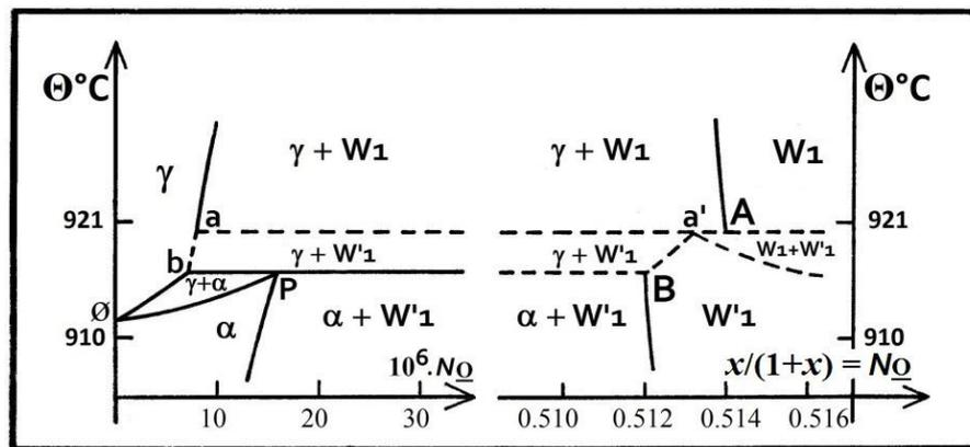
**Fig. 3. Equilibrium diagram ( $\text{FeO}_x$ ) between  $W1$  and  $W'1$  and ‘pure iron’, with both limit points  $A$  and  $B$  of  $\gamma\text{-Fe}/W1$  and  $\alpha\text{-Fe}/W'1$  boundaries. Compositions  $N_{\underline{O}} = x/(1+x)$  are arbitrarily taken at 1184 K in paper [28]. Dashed lines correspond with hypothetical limits.**
