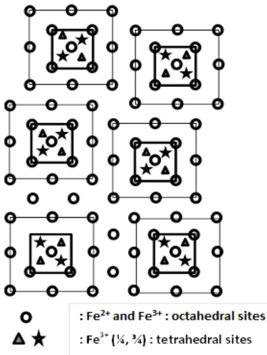
Fig. 18. Various orderings of clusters (10:4) in the fcc lattice of wüstite. The basic cluster can be the (13:4), the (10:4) or other possibilities with 4 interstitial sites occupied by cations  $Fe^{3+}$ . The disorder can develop by statistical displacement in one, two or three directions.  $2.55a$  could be the smaller inter-cluster distance ( $a$  = cell parameter of the “FeO” lattice).
