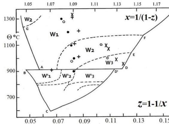
**Fig. 10:** Some determinations of the p-n transition by thermal e.m.f.. X: Geiger *et al.* [66] not corrected for platinum ; +: Bransky and Tannhauser [102]; ⊙ : Lafollet and Duquesnoy [104] by modeling; ○: Hillegas jr and Wagner jr [105]; ● : Gartstein and Mason [106] by re-examination of Hillegas jr’s thesis [82].
