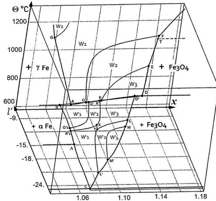
**Fig. 4. Phase diagram  $\Theta$  °C ( $l'$ ,  $x$ ) of solid wüstite  $FeO_x$  under equilibrium following Raccah-Vallet-Carel; upper temperature 1250 °C, lower one 592 °C at point C; coordinate  $l'$  for  $\log_{10}p(O_2)$ . Points noted by a capital letter are tabulated in [27], except the point  $\Lambda$  in [28] and the point T in [62] [63] [64].**
