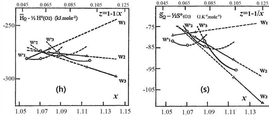
**Fig. 6.** Partial molar enthalpy ( $\bar{H}_O - \frac{1}{2}H^0(O_2)$ ) and entropy ( $\bar{S}_O - \frac{1}{2}S^0(O_2)$ ) of solution of oxygen, through the stability field of wüstite, whatever the temperature. Transitional jumps are at 820 °C (W'i) and 1000 °C (Wi). Dashed lines are drawn in extrapolated or metastable zones.
