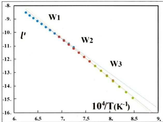
**Fig. 2. Variation of  $l'$  vs  $1/T$  for a fixed value  $z = 0.115$ : three quasi linear correlations corresponding to the initial determinations in the three domains W1 (high T), W2 (intermediate T) and W3 (low T) give rise to three activation energies  $\Delta H_i$ .**
