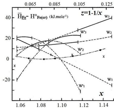
**Fig. 7.** Variations of the partial molar enthalpy ( $\bar{H}_{Fe} - H^0_{Fe}$ ) vs  $x$  for the isotherms at 1000 °C (Wi) and 820 °C (W'j). For comparison: ●---●:  $\Delta\bar{H}_{Fe}$  from e.m.f. measurements at 1000 °C by Asao *et al.* ([69] Table 3 p. 75); x: Darken and Gurry determinations ([31] Table X p. 1408).
