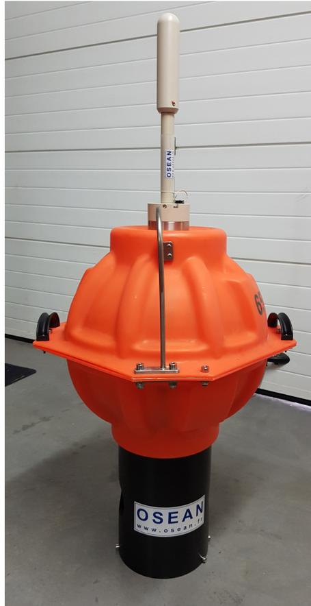
**Figure 6.** Bombyx2 - Project Interreg Maritime GIAS (whale anti-collision sonobuoy), here presented with communication antenna (4G or Iridium antenna) but without the acoustic 5 hydrophones antenna. The complete Bombyx2 is co-designed by LIS DYNi and IM2NP laboratories, SMIoT platform, OSEAN company.
