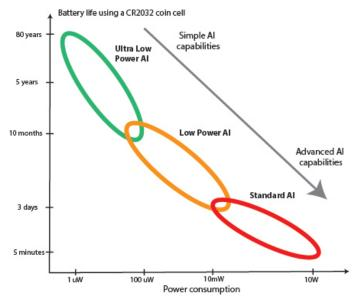
Figure 5. Different types of embedded AI according to their power consumption
