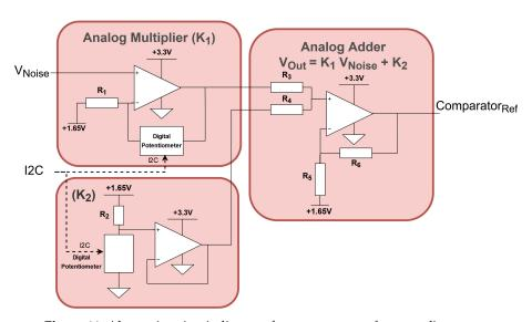
**Figure 11.** Alternative circuit diagram for comparator reference adjustment.
