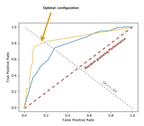
**Figure 15.** Click detector ROC curve using the state machine and expert rules validation (in yellow), versus without it (in blue) for different values of  $K_1$  parameter. Area under the ROC curve is 85% using the state machine and expert rules, versus 75% without.
