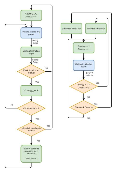
**Figure 14.** Cetacean click detection state machine (left), and automatic gain control state machine (right).
