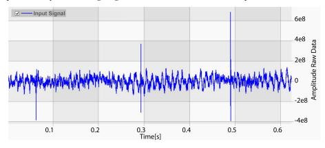
**Figure 9.** Cetacean click signal in output of the charge amplifier. Three clicks are present in the signal as well as sea noise.
