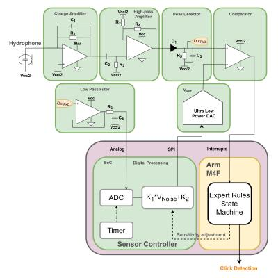
**Figure 8.** Electronic circuit of the always-on wake-up. ultra-low power parts are in green, low-power digital parts are in yellow. Voltage regulator and 1.65*V* reference are not presented.
