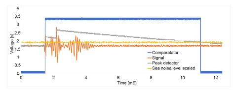
**Figure 12.** Real cetacean clicks and analog detection algorithm waveforms. High-pass filtered input signal is in orange,  $V_{Ref}$  in yellow, click envelope in grey and comparator output in blue.
