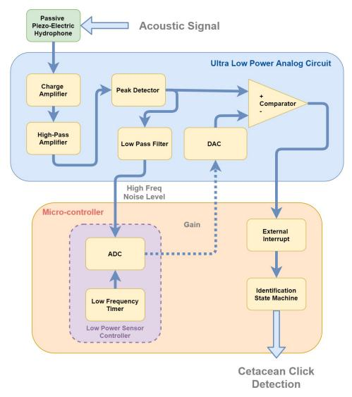
Figure 7. Sperm Whales detector block diagram.
