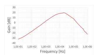
Figure 10. High-pass active filter measured frequency response.
