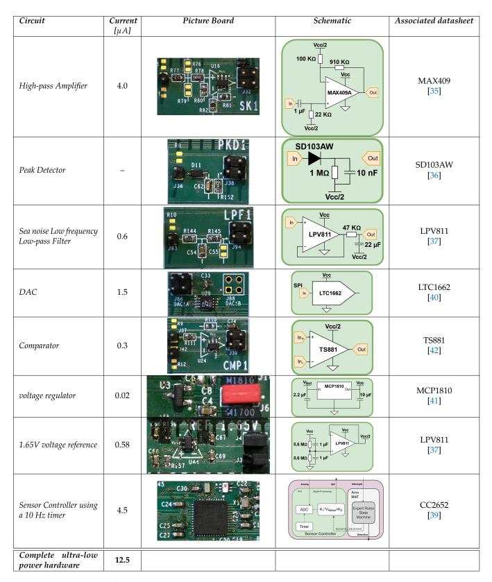
**Table 2.** Always-on ultra-low power analog circuits implementation and power consumption ( $\mu A$ ).
