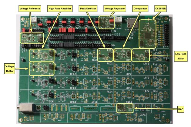
Figure 13. Analog test and power measurement board.
