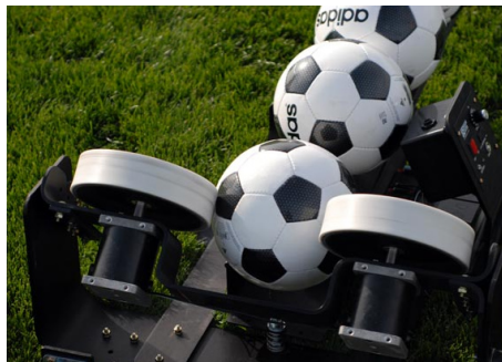
Figure 5. Mechanical inertial rotating launcher
