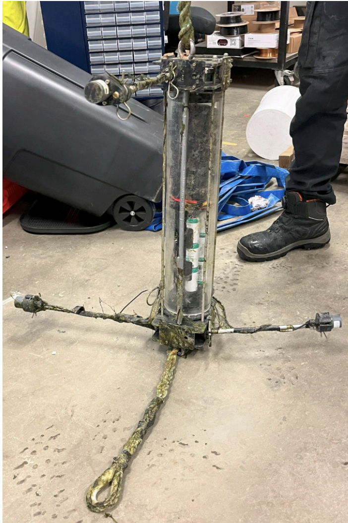
Figure 4.7 : BOMBYX3 DYNI LIS CNRS quadrasonic buoy, before and after deployment (november 2024 to June 2025), resulting from the know-how of the FEDER GIAS and ETHAC REGION SUD long autonomy program. These four hydrophones allow calculation of the bearing in azimuth and elevation of the sources, or even their distance, for detailed monitoring of wildlife over the long term. It was placed north of Haudoya Island, replacing the prototypical test buoy in the area placed (in stereo version) in our 2022 mission, but destroyed when it was taken over by a ship. It was rebuilt into 4 tracks and laid in November 2023 and successfully uploaded in January 2024.
