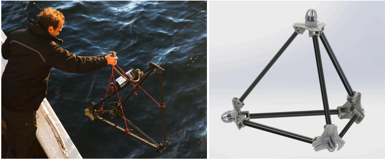
Figure 4.3 : (Left) Launching from Isbjorn II (photo credit Gies) of the tetrahedral antenna, equipped with its sound card and four hydrophones, designed by SMIoT LIS IM2NP UTLN (Right).
